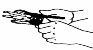
Extended position Note: Pressure, when handle is squeezed, holds adapter firm. Will not slip back.
